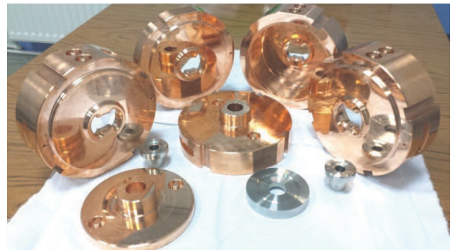
Figure 4: Parts of the cavity after machining, CANDLE SRI.
