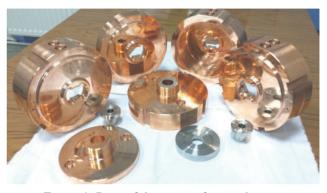
Figure 4: Parts of the cavity after machining.
